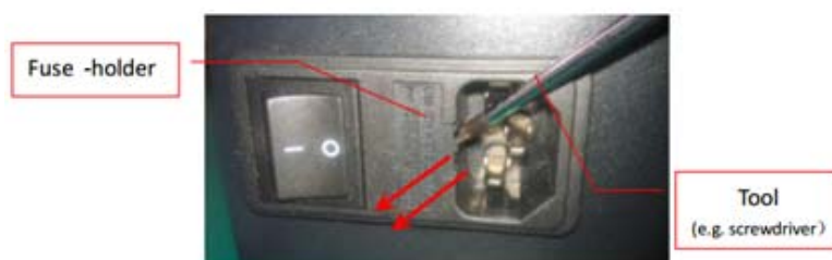
Fig 7.1 Remove the fuse holder from the power filter
